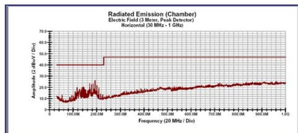
**Figure 1c: Horizontal Scan of 4-layer Model 2 in "Idle" Mode, Highest Peak ~ 26dB $\mu$ V**
