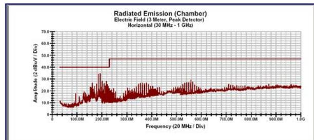
**Figure 1b: Horizontal Scan of 2-layer Model 2 in "Idle" Mode, Highest Peak ~ 34dB $\mu$ V**
